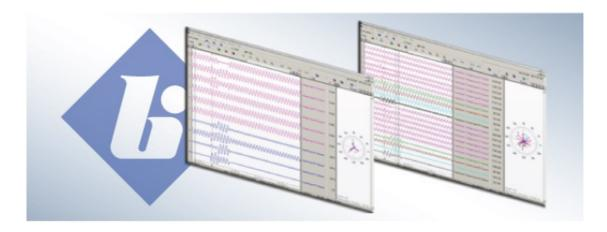
Wavewin Bitronics software allows for management, viewing and analysis of all Comtrade files from the 70 Series devices including those cross-triggered via GOOSE messaging). It can merge or append common files to create a single view and includes several analysis tools. The software permits the conversion of file names to the IEEE long file naming format (C37.232). Computed Software Channels are also provided for advanced analysis.
